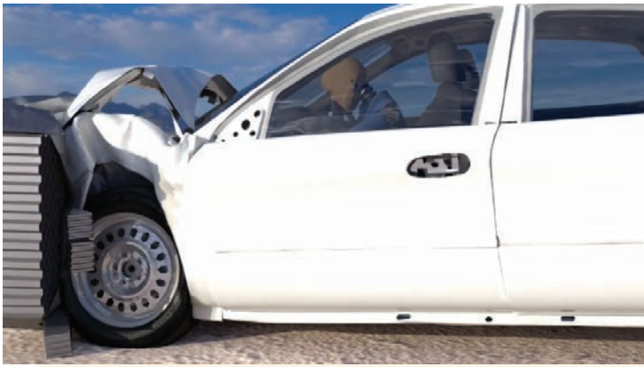
Figure 3: 3DEXCITE rendering of a Ford Taurus crash simulation using Abaqus. This model was developed by The National Crash Analysis Center (NCAC) of the George Washington University under a contract with the FHWA and NHTSA of the US DOT.
